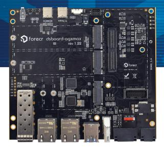
Introducing the DSBOARD-AGXMAX, the industrial carrier board that is built to maximize your productivity and connectivity. Powered by the high-performance AGX Orin SoM, which can deliver up to 275 TOPS of Al performance, this board offers top-of-the-line 10G connectivity, as well as Dual Gigabit Ethernet, USB 3.2, HDMI, CAN, Serial Ports, and MIPI CSI-2 Camera support.
