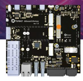
Introducing the DSBOARD-THRMAX, FORECR's most advanced carrier board purpose-built for the groundbreaking NVIDIA Jetson T5000 platform. With a powerful 128GB LPDDR5X memory interface, high-speed PCIe Gen5 storage, and a wide array of I/O options including dual HDMI 2.1, 1x DP 1.4a, USB 3.2, QSFP+, and robust serial connectivity, this compact 140x125mm board is engineered to support the most demanding edge AI applications.
