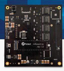
MILBOARD-XV is a carrier board designed for harsh military and aerospace environments. It is powered by the NVIDIA Jetson AGX Xavier module, which has an NVIDIA Volta GPU and an eight-core ARM64 CPU, providing high processing power for complex applications. The carrier board features a rugged design that ensures reliable performance even in the most extreme conditions. It has a wide operating temperature range and a robust power management system that can handle input voltages from 18V to 32V.
